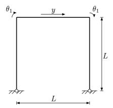
(b) The beams 1–3 and 2–4 are rigid, the remaining members of equal second moment area. Insert values of the elements  $k_{ij}$  in the equation  $\mathbf{P} = \mathbf{K}\mathbf{y}$ , where y is the vector of node translational displacements  $[y_1, y_2]$  and  $\mathbf{P}$  the corresponding horizontal forces.
