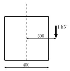
Determine the total strain energy in the cantilever. What proportion of the total deflection of the load is due to non-torsional shear strains and how would this proportion vary if the cantilever had a length of 1 m?
