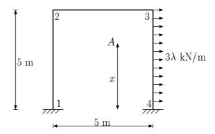
Now assume a mechanism with plastic hinges at sections 1, 2, 4 and *A*, retaining *x* as a variable. Show that in the actual collapse mechanism x = 3.66 m, and that  $\lambda_c = 1.194$ .
