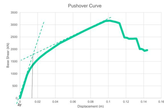
Pushover is used to determine the response of a structure under permanent vertical forces and general increasing horizontal forces. From the curve:
