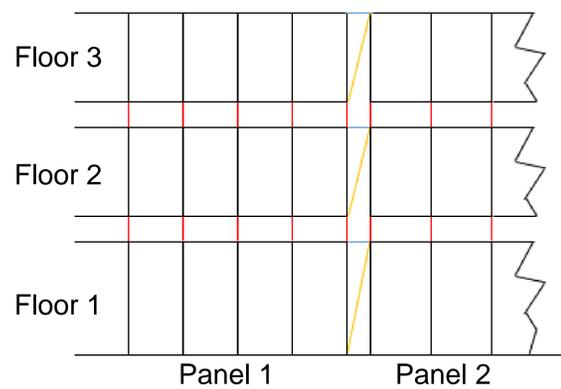
The figure shows how the floors and panels are connected in the model. The gaps between panels and floors are all  $1 \times 10^{-5} m$ .
