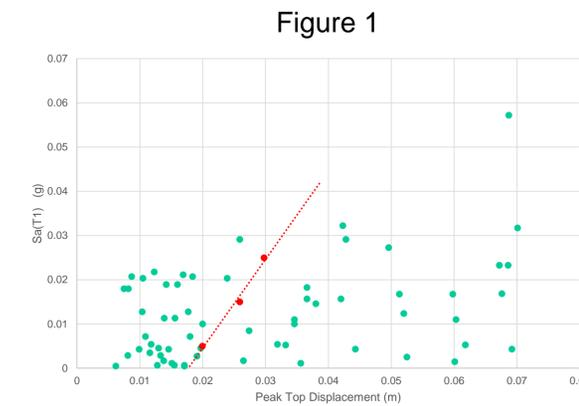
Figure 1 is the relationship between Spectral Acceleration (SA) and the Peak Top Displacement of the structure. Each green point represent one earthquake, red dots is the mean value of the logarithmic number of the displacement in every intervals, here the intervals are 0.01 at y-axis.
