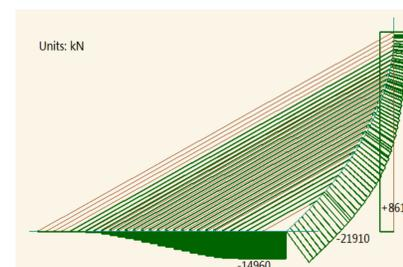
Figure 5: Axial force distribution of the benchmark model under a live load of 100 kN/m
