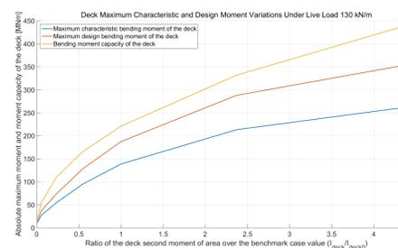
Figure 9: Moment capacity check for the deck
