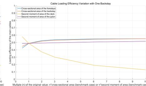
Figure 7: Cable loading efficiency variation
