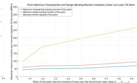
Figure 10: Moment capacity check for the pylon
