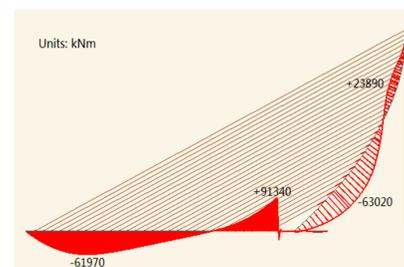
Figure 4: Bending moment distribution of the benchmark model under a live load of 100 kN/m
