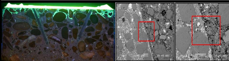
Slag samples appeared to be the most dense while For fly ash, as the particles are spherical and in the same size range as Portland cement, it reduced the permeability of concrete. The ground cementitious spacers were observed to have less penetration in the silica fume samples compared to the fly ash samples.
