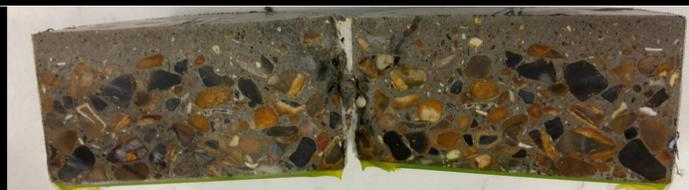
Following this, further sectioning of the fly ash samples into 20mm x 40mm x 8mm blocks was carried out, which were required for Backscattered Electron microscopy. The cementitious spacer was also studied using the BSE microscope for comparability and to provide further insight on its microstructure and properties.
