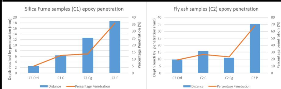
Analysis was carried out using ImageJ. In all cases the plastic spacer accommodated the most penetration along its boundary, reaching a maximum of 67% of the sample height. The images were segmented and thresholded using the fluorescence of the epoxy in order to calculate the fraction of the total volume that is occupied by epoxy.
