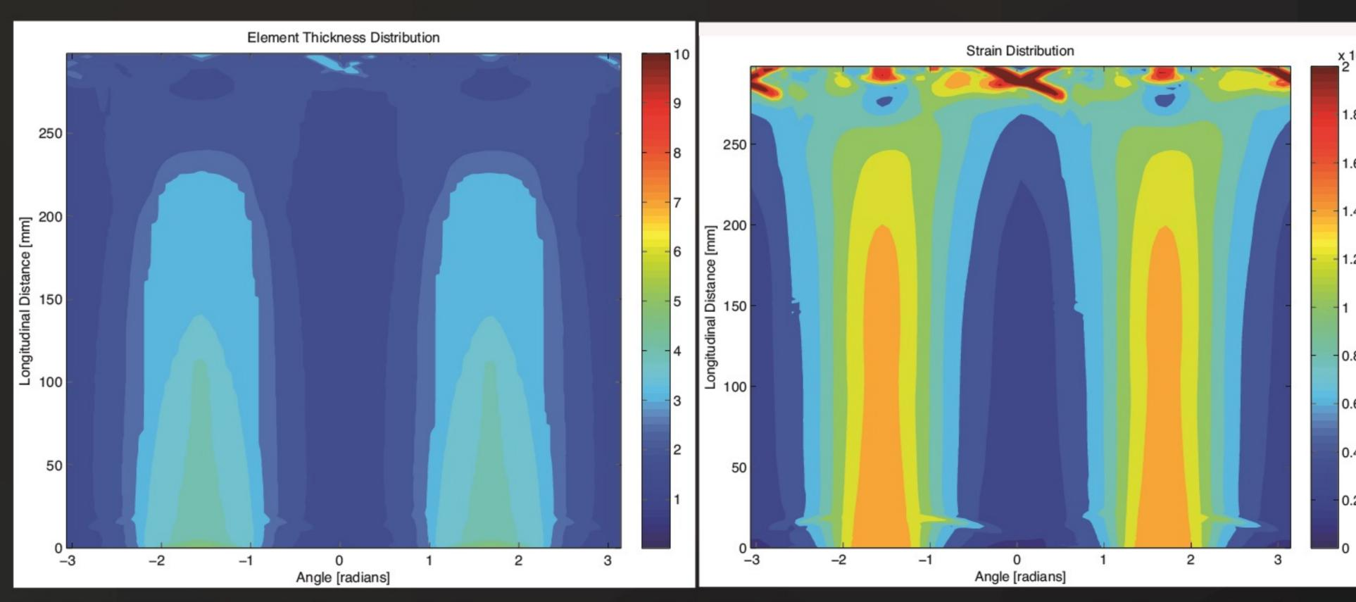
Thickness variaion of elements within the structure; and the strain distirubtion in the structure.
