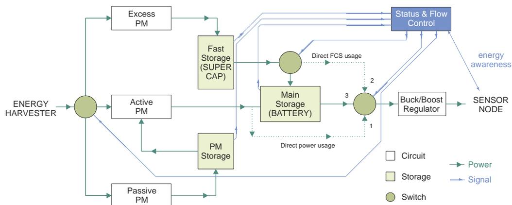
**Figure 4.** Block diagram of an example hybrid storage architecture with dynamic power routing control for portable power supplies. energy harvesting systems. This system includes a battery main storage, a super-capacitor high-power storage (FCS) and a separate storage unit for passive power management.
