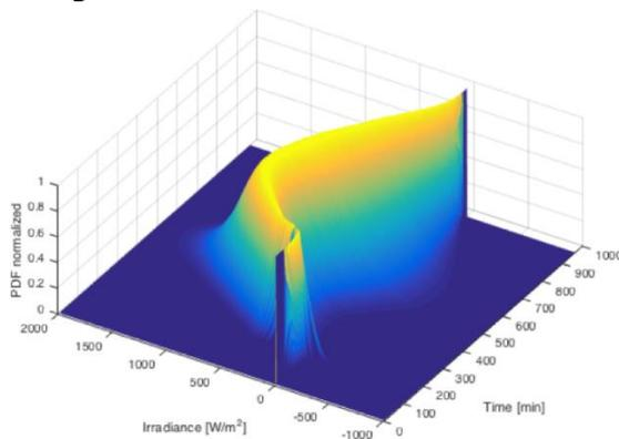
**Figure 2.** The probability density function of solar input to a Simulink Model. The data represent 13.8 years of solar irradiance from the National Renewable Energy Lab station in South Park, Colorado, USA.
