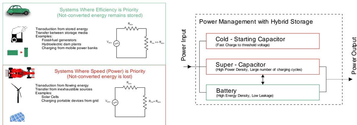
**Figure 1.** Left: Illustration of the difference between cases where maximization of efficiency or net power transfer is more important. Right: Block diagram of the proposed hybrid energy storage architecture for portable systems.
