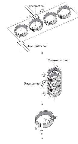
**Fig. 1** Schematic presentations a Planar configurations with measuring coils b Axial configurations with measuring coils c Dimensions of the split ring
