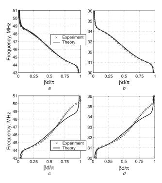
Fig. 2 Dispersion characteristics of arrays consisting of identical elements
