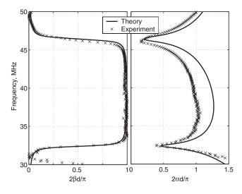
**Fig. 3** Dispersion characteristics for a bi-periodic planar array a Propagation constant b Attenuation constant
