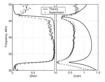
**Fig. 4** Dispersion characteristics for a bi-periodic axial array a Propagation constant b Attenuation constant
