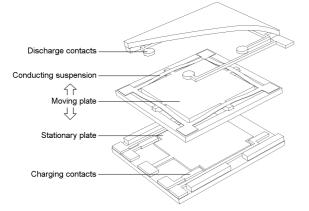
**Figure 4** MEMS Electrostatic energy scavenger for low frequency applications (from [7]), using a Si proof mass on a polyimide suspension.
