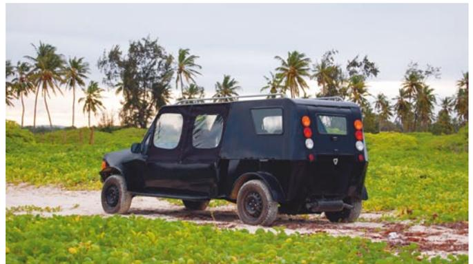
**Four-wheel drive, a tough, tubular steel frame at an auto rickshaw price – the prototype Mobius One.**
