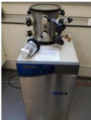
Freeze-drying is a drying process, where the solvent (normally water) is eliminated from the sample via direct sublimation from solid to gas phase. This is a useful way of eliminating solvents by keeping the material structure intact for further processing, like for example sintering.
