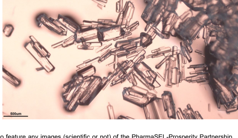
Figure 4. Glycine crystals obtained during cooling crystallisation experiments.
