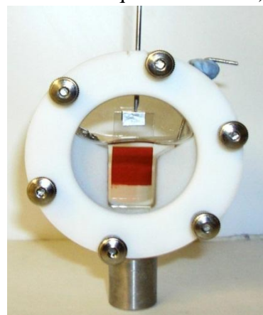
Figure 2-1. Picture of the three-electrode cell.
