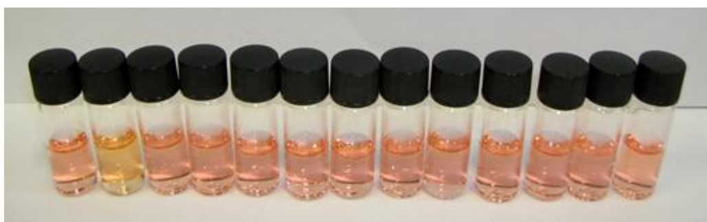
Figure 4-2. Color changes observed by “Naked Eye” at 12.5 μM M + ions (for Hg 2+ is 2.5 ppm) aqueous solution as 2 mM N19/ethanol solution added. From left to right: No metal ions, +Hg 2+ , +Ca 2+ , +Mg 2+ , +Fe 3+ , +Fe 2+ , +Cd 2+ , +Cu 2+ , +Co 2+ , +Ni 2+ , +Pb 2+ , +Zn 2+ , +Li + .
