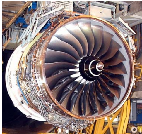
Fig. 3-5. Trent 1000 fan ran for the first time on 14th February 2006
