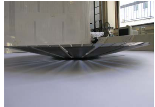
Fig. 4-5. Swept Blisk 15deg (after second bending)
