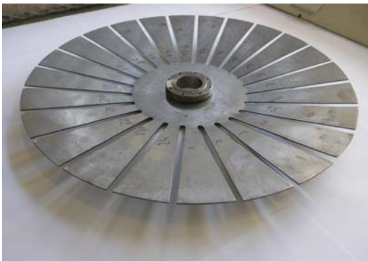
Fig. 4-5. Swept Blisk 15deg (after second bending)
