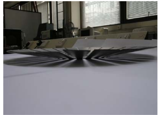
Fig. 4-4. Swept Blisk 10deg (after first bending)
