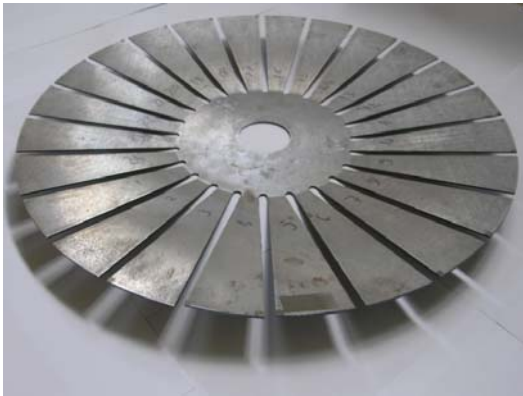
Fig. 4-4. Swept Blisk 10deg (after first bending)
