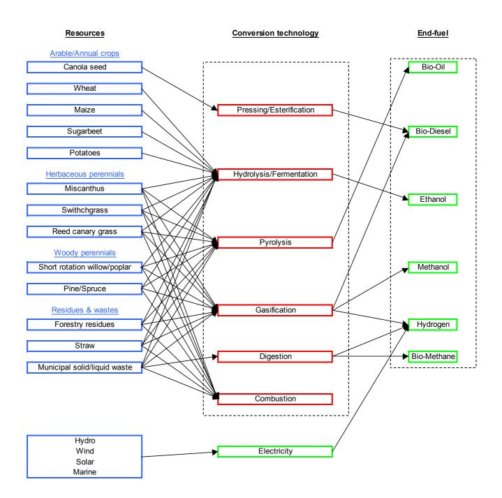
The fuel sources or 'Resources' shown in this diagram represent those available in the UK. 'Conversion Technologies' and 'End-Use' sections apply internationally.
