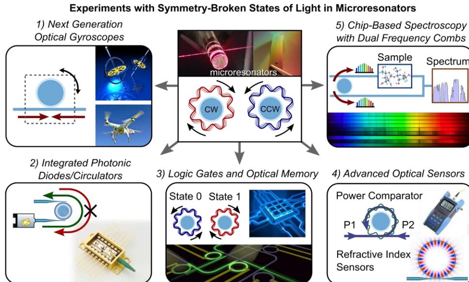
**FIG. 1:** Illustration of future applications for symmetry-broken states of light in microresonators.
