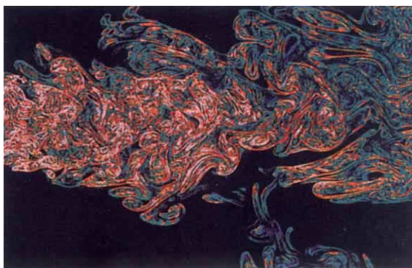
Section through a turbulent water sheet, visualized with fluorescing dye and laser sheet (a plane of laser light). Reprinted from ref. 13.
