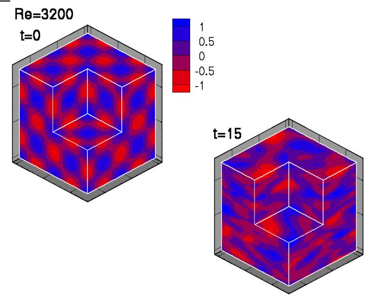
Three-dimensional contour plots of the stream function for the case with  $F_{\ell} = 4$ ,  $R_{\ell} = 3200$  at t = 0 (left) and t = 15 (right).
