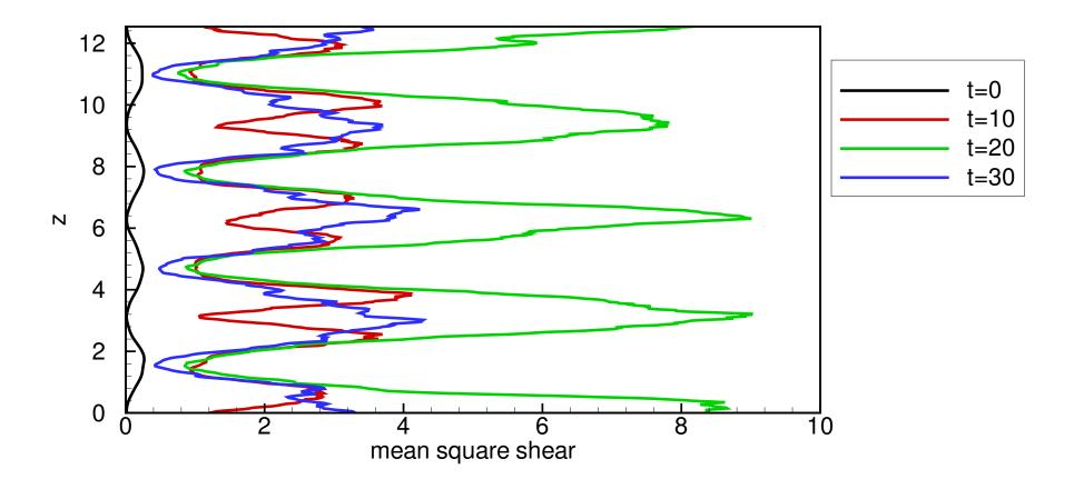
Mean square vertical shearing of the horizontal velocity vs z.  $F_{\ell} = 4$  and  $R_{\ell} = 6400$  at different times.
