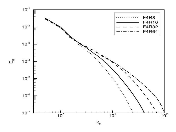
Horizontal kinetic energy spectra at t = 20 for four different  $R_{\ell}$  cases.
