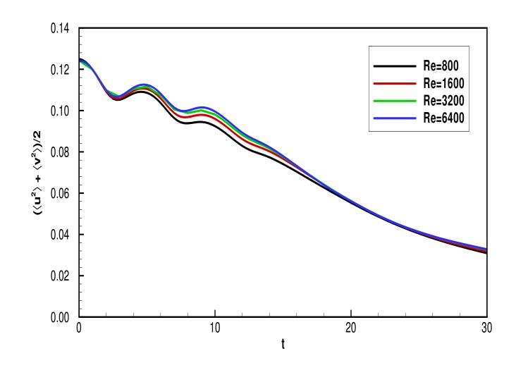
Volume-averaged horizontal kinetic energy vs t,  $F_{\ell} = 4$ , various  $R_{\ell}$ .
