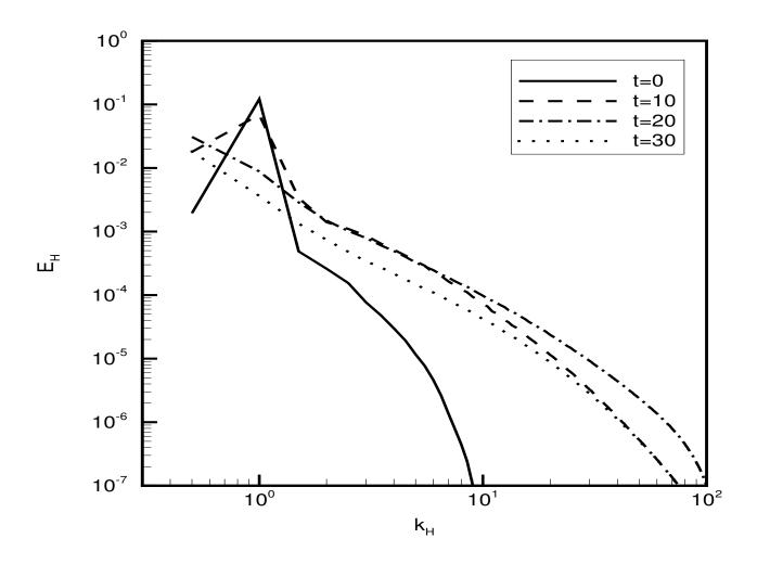
Horizontal kinetic energy spectra at t = 0, 10, 20, 30;  $F_{\ell} = 4$ ,  $R_{\ell} = 6400$ .
