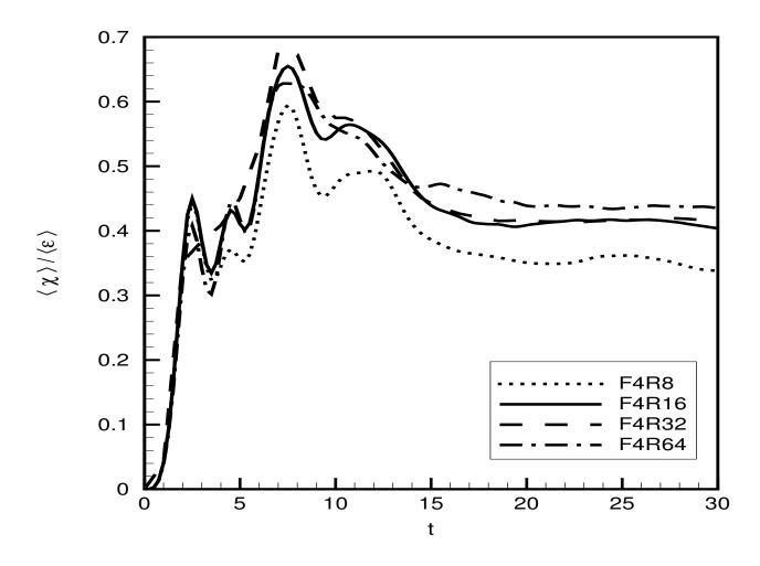
Mixing efficiency vs t,  $F_{\ell} = 4$ , various  $R_{\ell}$ .
