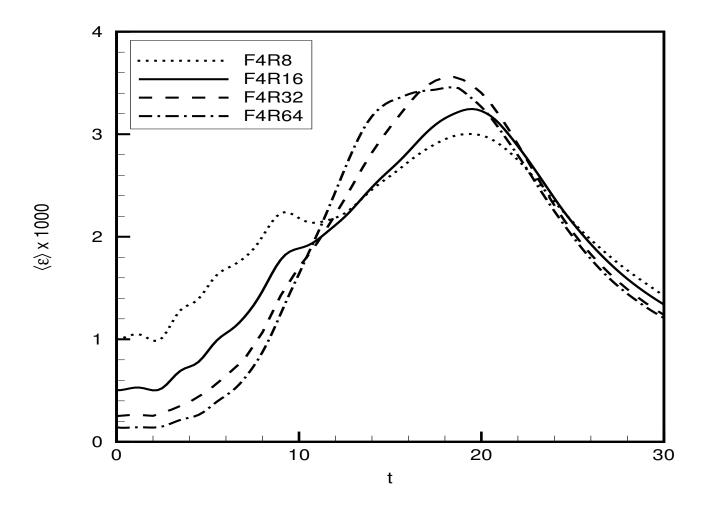
Volume-averaged kinetic energy dissipation rate vs t,  $F_{\ell} = 4$ , various  $R_{\ell}$ .
