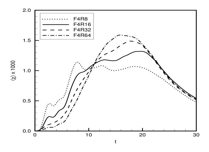
Volume-averaged potential energy dissipation rate vs t,  $F_{\ell} = 4$ , various  $R_{\ell}$ .
