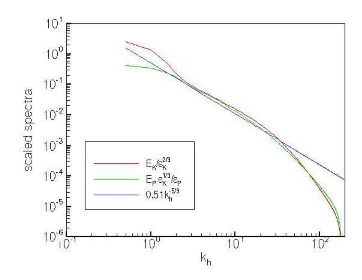
Horizontal kinetic energy spectra at t = 18.5 for  $R_{\ell} = 9600$  case.
