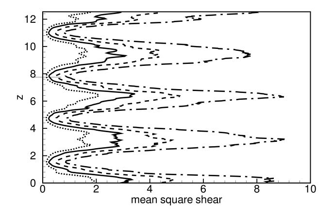
Mean square vertical shearing of the horizontal velocity vs z.  $F_{\ell} = 4$  and t = 20 for  $R_{\ell} = 800, 1600, 3200, 6400$ .
