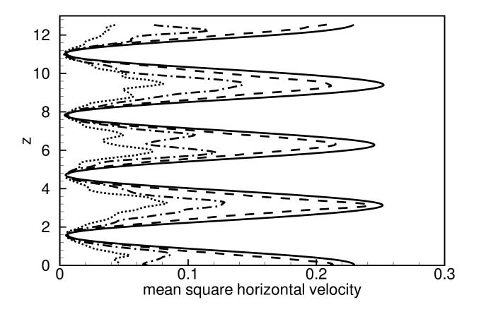
Mean square horizontal velocity vs z.  $F_{\ell} = 4$  and  $R_{\ell} = 6400$  at t = 0, 10, 20, 30.
