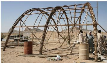
Known for his keen interest in evidence-based eco-technology, His Highness observed testing of palm leaf structures using rigs normally applied to steel.
