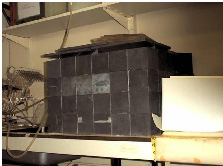
This picture shows a lead 'castle' which was constructed on a bench top. Whilst the user thought they were doing the right thing, the actual amount of lead used far exceeded the shielding requirements (its use was not ALARP<sup>5</sup>). The lead shielding had a mass of at least 300 Kg, which was most likely overloading the bench.
