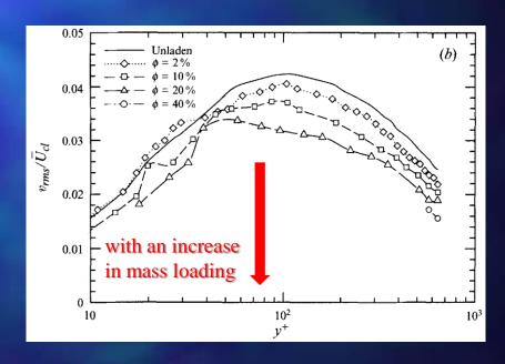
Turbulence modulation by solid particles
