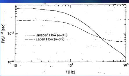
Turbulence modulation by solid particles
