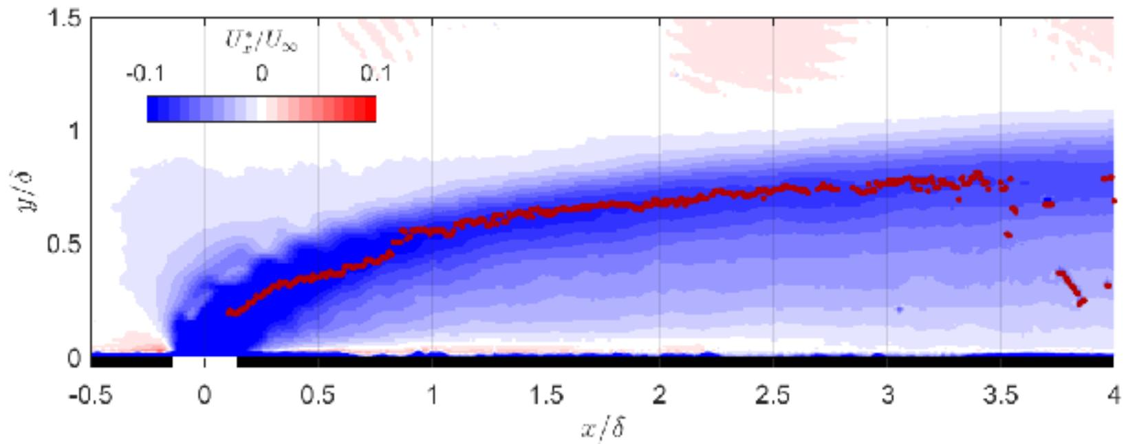
Trajectory measured from hot-wire measurements matches PIV
