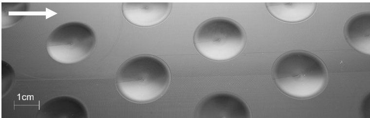
Photograph of A-configuration test plate which reduces turbulent skin friction drag
