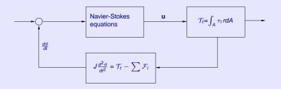
Freely rotating discs can be seen as a feedback system
