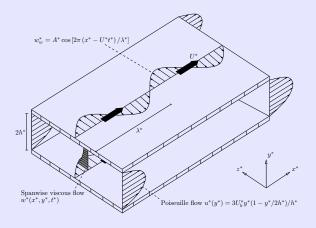
We did some work on laminar wave flow  $\to$  but Stokes layer was assumed thin  $\delta \ll h$  But interesting flow features may occur when  $\delta = \mathcal{O}(h)$
