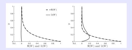
WKBJ asymptotic solution and numerical solution match ...but NOT valid for  $U_{waves}$  close to  $U_{bulk}$
