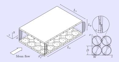
First proposed by L. Keefe (1998), but no results Fully-developed turbulent channel flow  $R_{ au}=$  180 - DNS: x,z Fourier, y Chebyshev Parameters: D diameter, W maximum tip velocity
