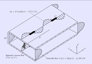
Spanwise laminar flow can be used to study drag-reduced turbulent flow
