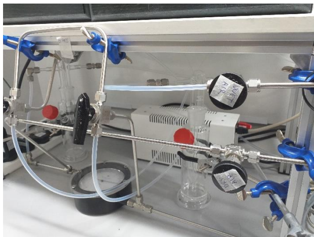
Figure 8. The two dreschel bottles (one dry; one filled with distilled water just above the inlet), hygrometer and two needle valves for creating humidity inside the reactor
