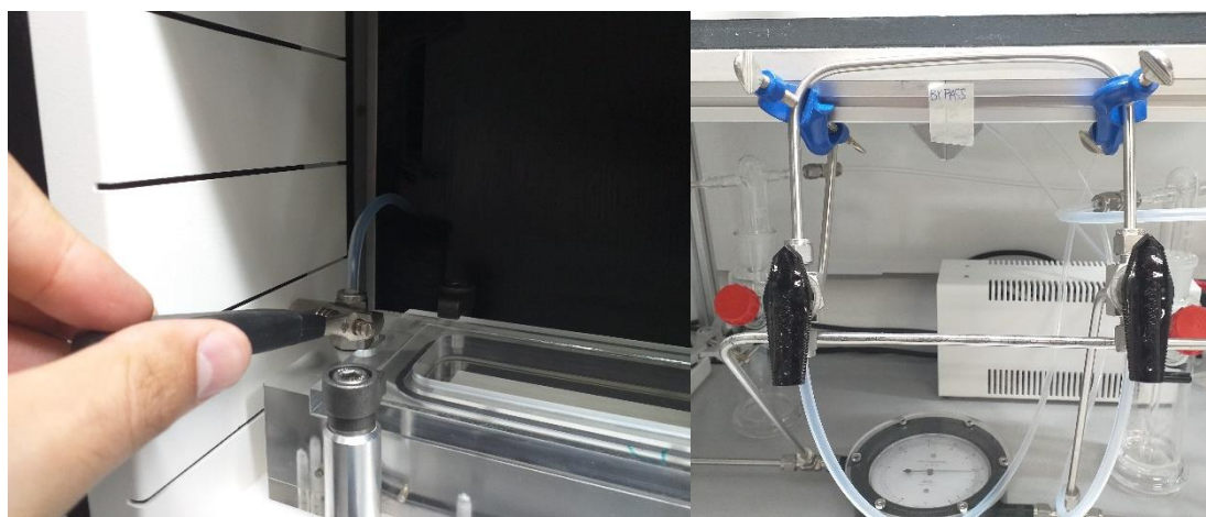
Figure 7. How to remove the reactor from the black cupboard (left), and the by-pass valves (right)
