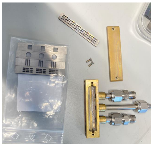
Inside the baffle manifold (perforated steel plates, etc.)
