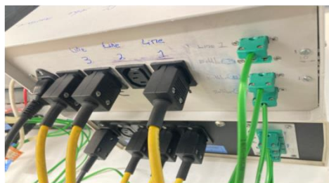
back side of heating line temperature control box and bubbler temperature control box
