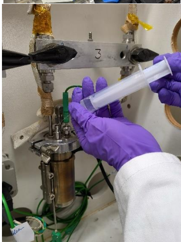
Bubbler Injection with N 2 Protection
