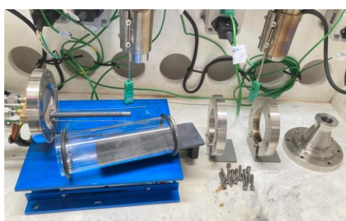
CVD reactor disassembled and carbon block removed
