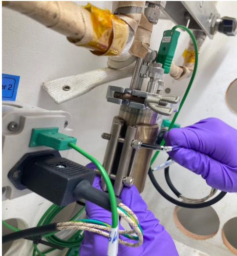
loading/ unloading precursors in bubbler
