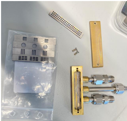
Inside baffle manifold
