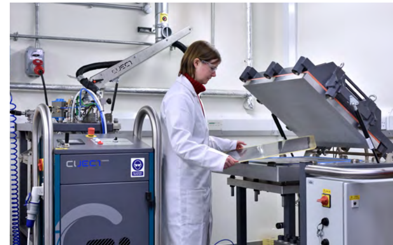
▲ Out of autoclave manufacture of composite laminates.
