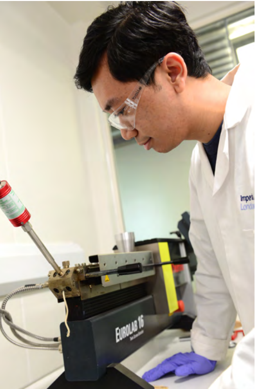
▲ Extrusion of thermoplastic polymer.
