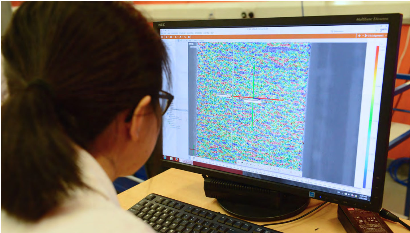
▼ Digital Image Correlation of notched composite.
