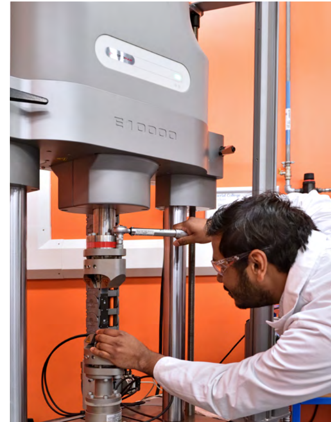
▲ ElectroPuls electrodynamic mechanical test machine
