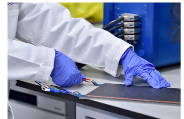
▲ Electrochemical testing of structural supercapacitors.
