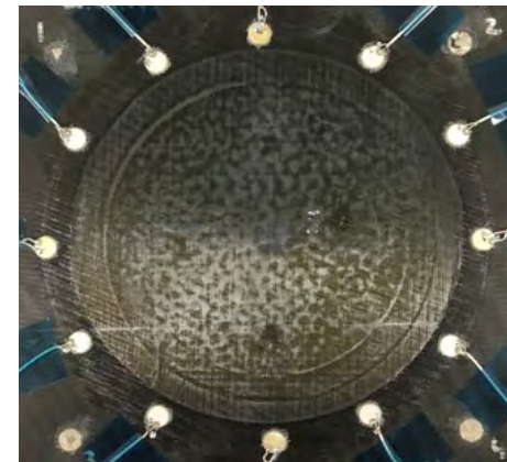
▲ Instrumented repair of a composite aerostructure.
