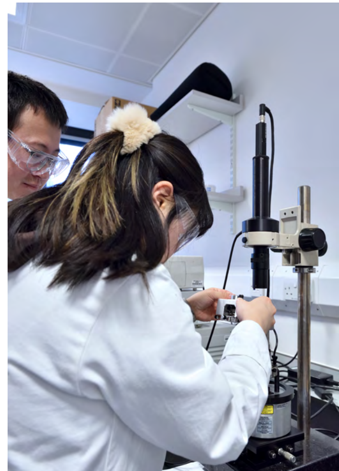
▼ Atomic Force Microscope examining nanocomposites.
