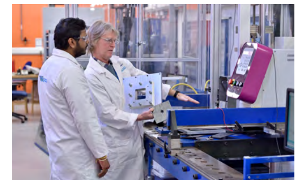
▲ Impact testing of CFRP.
