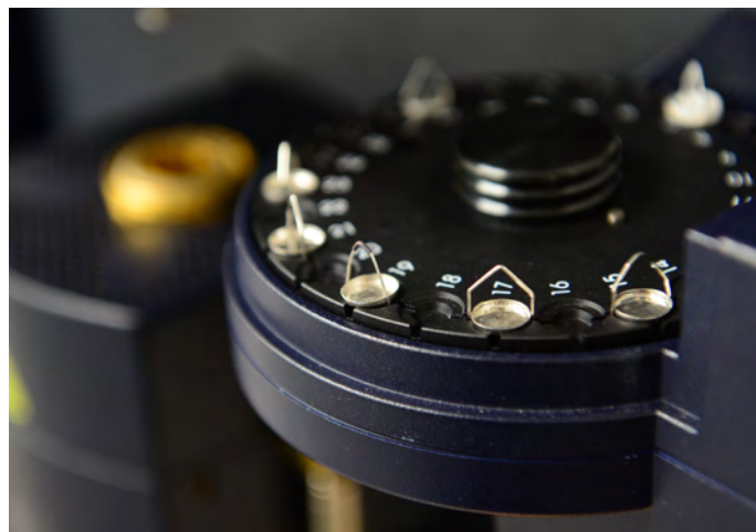
▲ Composite characterisation using ThermoGravimetric Analyser (TGA).
