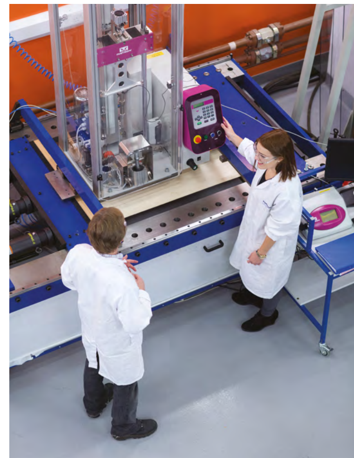
▲ Bespoke drop-weight impacted with compression frame to undertake impact whilst under loading.
