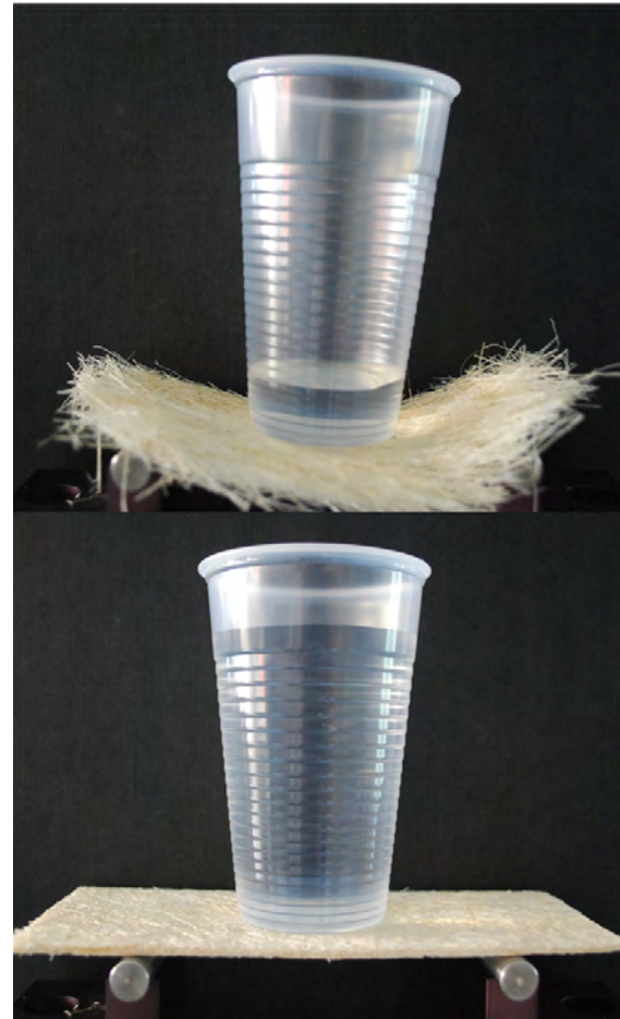
▲ Short sisal fibre composites without (top) and with (bottom) bacterial cellulose.
