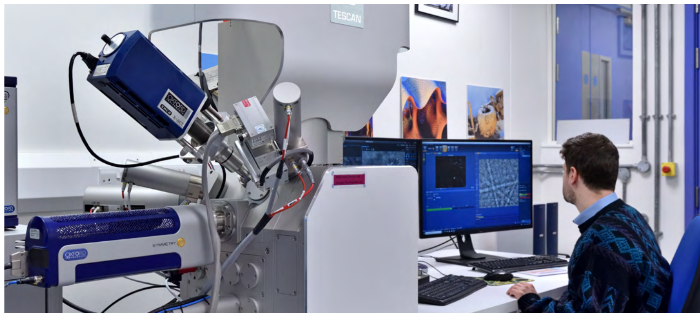
▲ FEG-SEM used for characterisation of composites.
