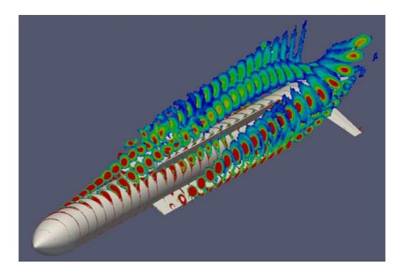
Fig 1: Image of vortex dominated flow field over generic missile configuration obtained using contemporary MBDA CFD tools.
