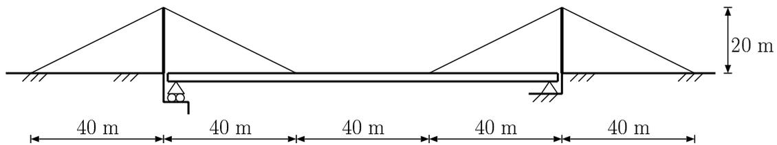
Evaluate the deflection at mid-span and at the points of attachment of the cables to the deck, due to a load of intensity
