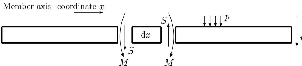
Displacement  $v$ , moment  $M$ , shear force  $S$  and load intensity  $p$
