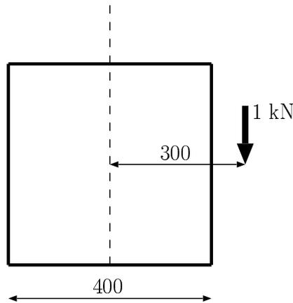
Determine the total strain energy in the cantilever. What proportion of the total deflection of the load is due to non-torsional shear strains and how would this proportion vary if the cantilever had a length of 1 m?
