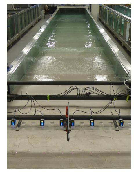
Hydrodynamics are scaled according to Froude scaling, which ensures fluid motion similarity between nature and the model (Hughes, 1993).
