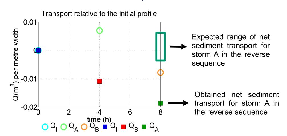
Overall, profiles exhibit greater variability and sediment transport rates when a more powerful event starts the sequence. Localised erosion due to onshore transport at the lower beach face occurs when waves pass the outer bar without breaking (Experiments 1 and 3). Waves reform along the trough and break at a further onshore position.
