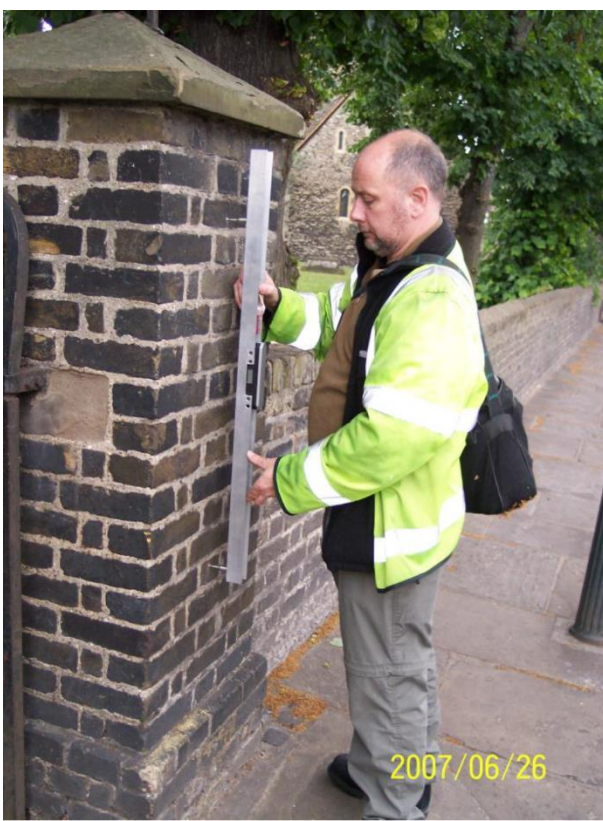
Figure 3: Taking a tilt measurement with inclinometer.
