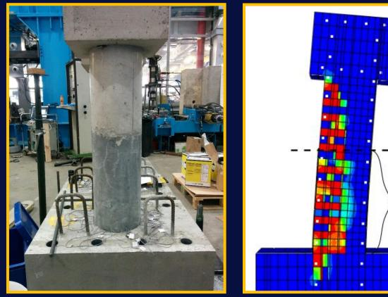
Seismic conditions have been reproduced statically by applying a constant vertical load and a displacement-controlled monotonic horizontal load [1]. The main reason behind the use of the steel tube on the half bottom of the column is that the confinement action can compensate for the strength loss due to rubber replacement. Additionally, steel tube confiment in the plastic hinge region produces some enhancement in ductility.
