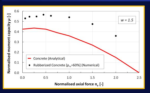
Unconfined RuC columns with  $\rho_{rv}$ =60% present larger  $\mu - n_v$  domain compared to an equivalent low strength concrete [2]. Conversely, there is a significant capacity reduction which is fully covered by the addition of the steel tube. While at low values of thickness, the column exhibits high ductility due to the contribution of the RuC core; the use of a stiffer tube produces the occurrence of concrete crushing at the mid-height ('weak section').
