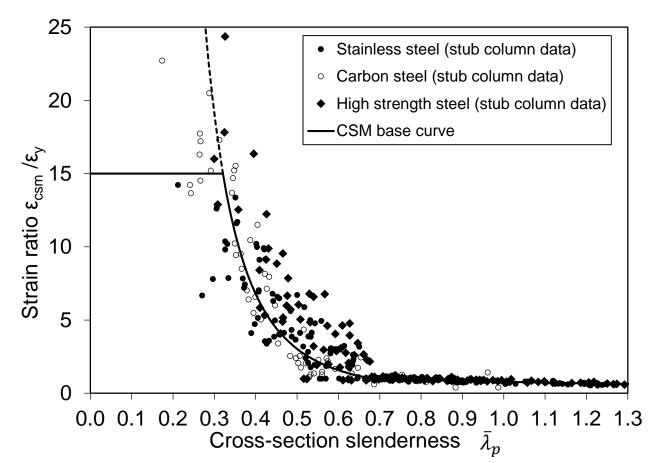
Base curve, based on stainless steel, carbon steel and high strength steel test data
