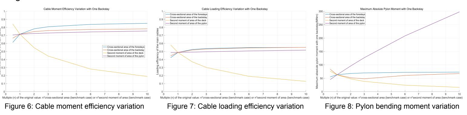
The impacts of increasing the number of backstays are also analysed. Having multiple backstays will increase both the cable efficiencies and the pylon bending moments. As a result, evidences are not enough to prove the resultant improvement in the overall structural performance of the bridge under live load.
