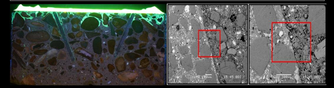
Slag samples appeared to be the most dense while For fly ash, as the particles are spherical and in the same size range as Portland cement, it reduced the permeability of concrete. The ground cementitious spacers were observed to have less penetration in the silica fume samples compared to the fly ash samples.
