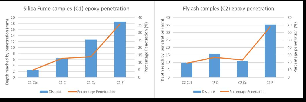
Analysis was carried out using ImageJ. In all cases the plastic spacer accommodated the most penetration along its boundary, reaching a maximum of 67% of the sample height. The images were segmented and thresholded using the fluorescence of the epoxy in order to calculate the fraction of the total volume that is occupied by epoxy.
