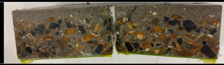
Following this, further sectioning of the fly ash samples into 20mm x 40mm x 8mm blocks was carried out, which were required for Backscattered Electron microscopy. The cementitious spacer was also studied using the BSE microscope for comparability and to provide further insight on its microstructure and properties.
