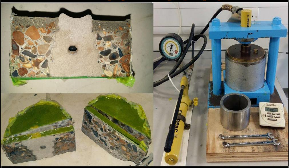
Struer's epoxy resin was used with a ratio of epoxy to hardener to toluene equal to 25:3:5%. The samples were placed in a pressure chamber set at 2.5 bars for 22 hours to accommodate for the penetration.. The samples were then sectioned in half and after drying each side was imaged under ultraviolet lighting after common noise reduction techniques were used, such as sonic bath in acetone and compressed air.
