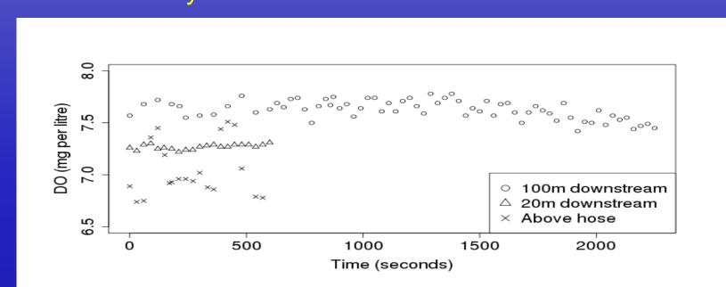
No changes in DO level after pumping air into water
