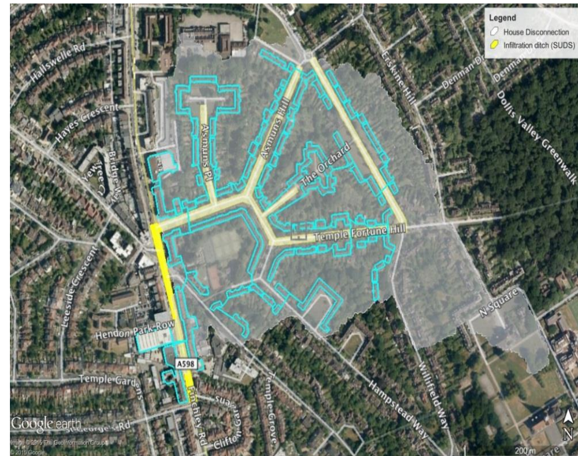
Figure 1: Police station sub-catchment showing the disconnection of roofs and implementation of SUDS
