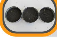
Obtained from pyknometer tests. HPF5 2.67
