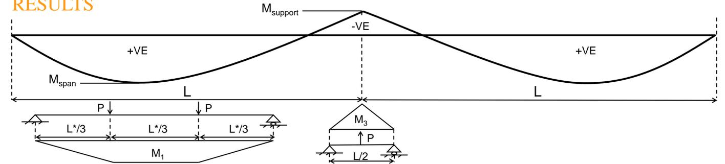
Figure 4: Elastic bending moment diagram
