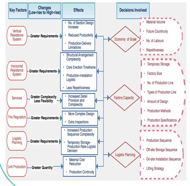
Complexity and risk can be induced from low-rise to high-rise light steel frame modular when considering all listed factors in the **Decision Network. Decision** and preparation are more time-consuming when accounting for all effects. The pre-construction planning for high-rise light steel frame module is based on an analysis of all the factors discussed above as well as by incorporating opinions from experts in industry.
