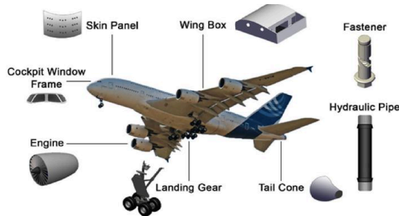
Figure 1. Example of the applications of titanium alloy used for an aircraft. [1]
