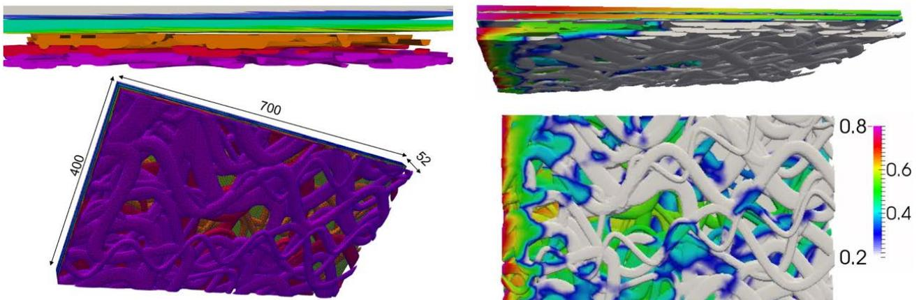
**Fig 1** : Top left figure shows the permeability map of a complex reservoir model. Bottom left figure shows the channel system of the reservoir from below. Top right and bottom right figure display the saturation field at different times seen from the side-below and from below, respectively.
