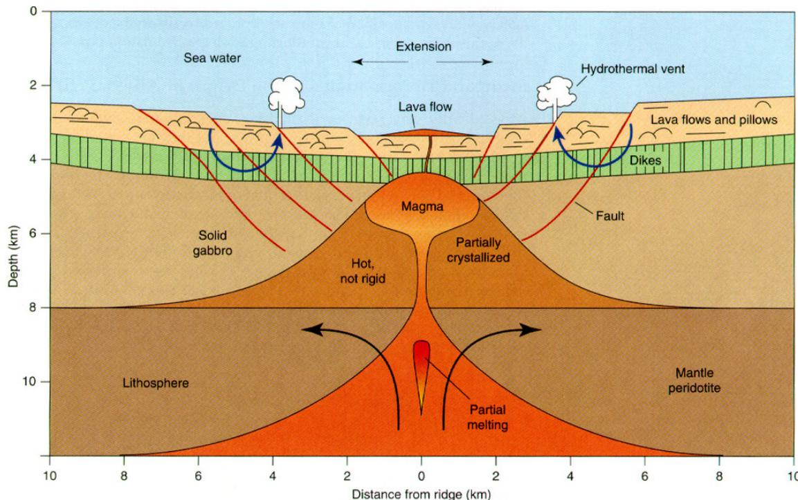
**Figure 1. Typical textbook image of a mid-ocean ridge. Geophysical imaging shows that the magma reservoir beneath the ridge comprises a liquid-poor 'mush' of crystals with melt present along grain boundaries. This project will investigate the fluid dynamics of such reservoirs.**
