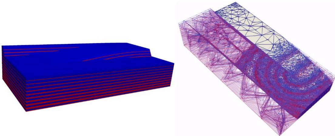
**Fig. 1:** Left: meshless heterogeneity blueprint coloured by permeability (red: high; blue: low) representing a relay ramp of a layered reservoir. Right: IC-FERST flow simulation showing optimized mesh of varying resolution coloured by wetting-phase saturation (red: high; blue: low). It can be seen how, the importance of an accurate representation of the geology could be variable across the domain.
