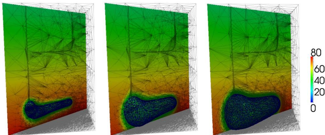
**Fig. 1:** Low enthalpy geothermal reservoir with a doublet system. The injector, (left well) introduces water at a lower temperature. The mesh is adapted as the low temperature water is being injected in the system: (Left) Adapted mesh, temperature field and isosurface at 36 C after 18 years production. (Centre) Adapted mesh, temperature field and isosurface at 36 C after 66 years production. (Right) Adapted mesh, temperature field and isosurface at 36 C after 110 years production.
