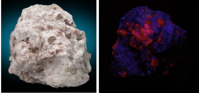
Zunyite in pyrophyllite and euhedral quartz, Big Bertha Extension, Dome Rock Mountains, La Paz County, Az (high sulphidation gold prospect). Hand specimen and sample under UV light showing pink zunyite fluorescence. John Betts Fine Minerals.
