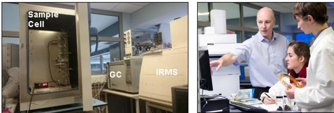
*Figure 1. The online shale adsorption/desorption cell-gas chromatography-combustion-isotope ratio mass spectrometry system at Imperial College London.*
