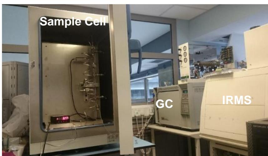
*The world's only online desorption cell-gas chromatography-combustion-isotope ratio mass spectrometry system at Imperial College London.*
