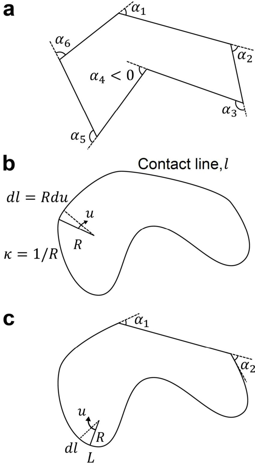
Figure 1. An illustration of angles and curvatures in two dimensions. (a) For a polygon the sum of the external angles  $\alpha_i$  is  $2\pi$ . Note that  $\alpha_4$  in a concavity is negative. (b) For a smooth closed loop the equivalent relationship is that the integral of the curvature around the loop is  $2\pi$ . (c) For a two-dimensional shape bounded by straight sides, sharp angles and smooth lines, the generalization of the relationship between curvature and angles is given by Eq. (1).
