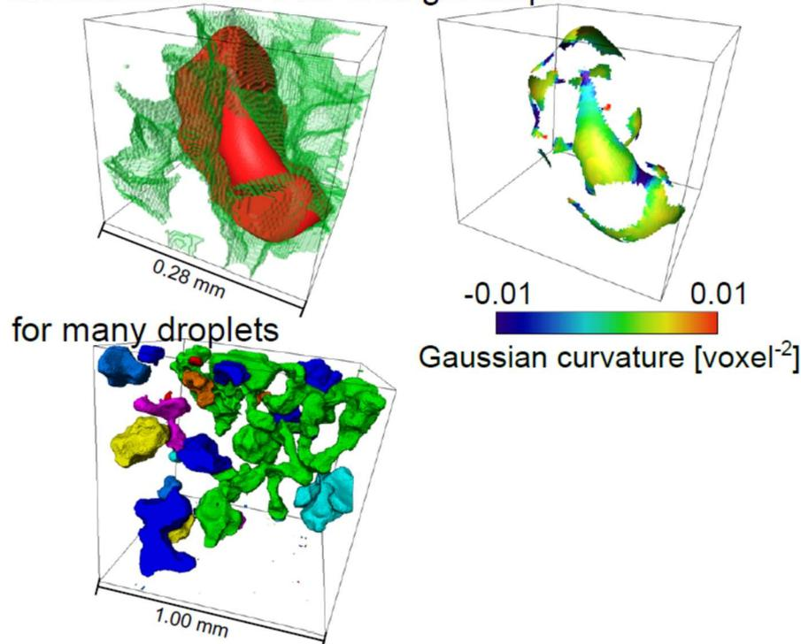
**Figure 3.** Pore-scale images of phases in a porous medium – the colours distinguish phases, distinct ganglia or the Gaussian curvature of the interfaces. These images can be used to quantify contact angle,  $\theta$ , using topological principles.
