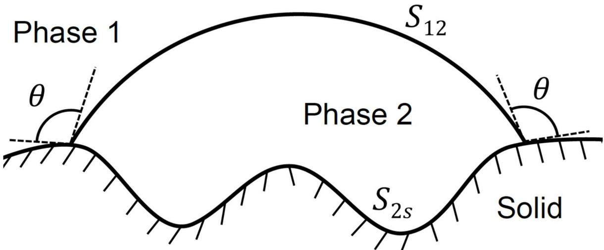
**Figure 2.** A schematic of a drop of phase 2 on a solid surface surrounded by phase 1. The contact angle  $\theta$  is shown. We can use Eq. (2) to relate the integral of the Gaussian curvature over the surface  $S_{12}$  to contact angle.
