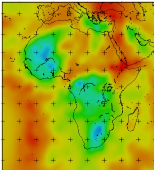
*An estimate of temperatures at 100 km depth below Africa determined from the surface wave velocities from Fischwick (2010).*
