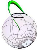
Fig. 4. Qualitative display of loaded resonator Q-factor in the normal plane of the differential-phase group delay curve given in Fig. 2, creating a generalized cylinder of radius proportional to (15).
